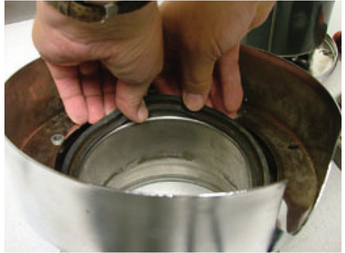
Figure 11. Replacing Shredder Gasket
