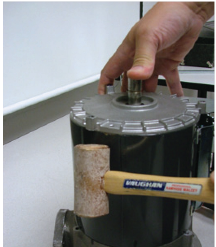
Figure 30. Marking and Removing Lower End Framer
