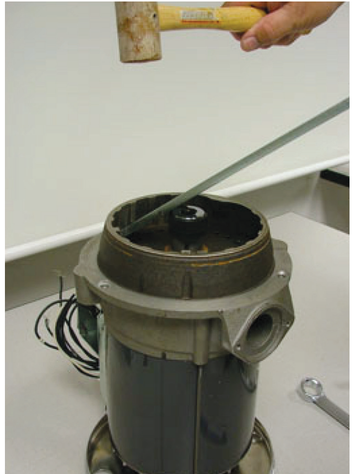
Figure 12. Removing Stationary Shredder
