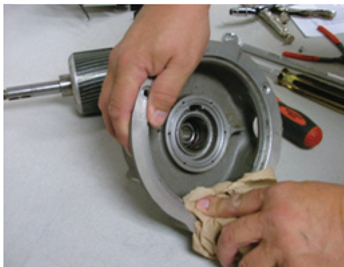
Figure 21. Cleaning Upper End Bell
