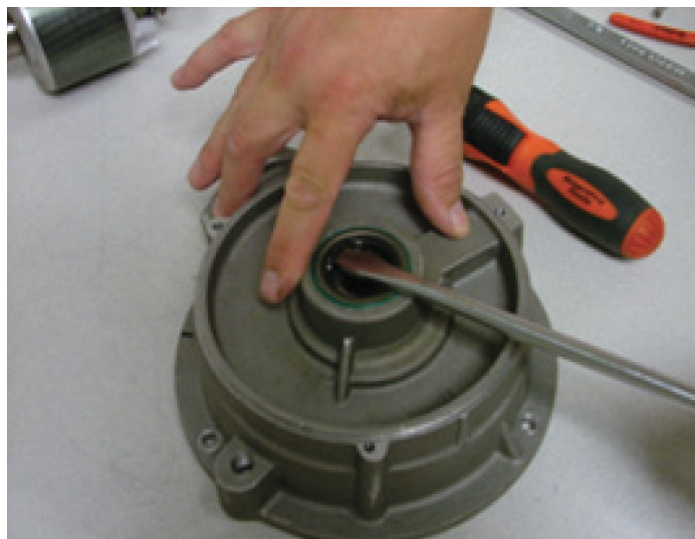
Figure 20. Water and Oil Seal
