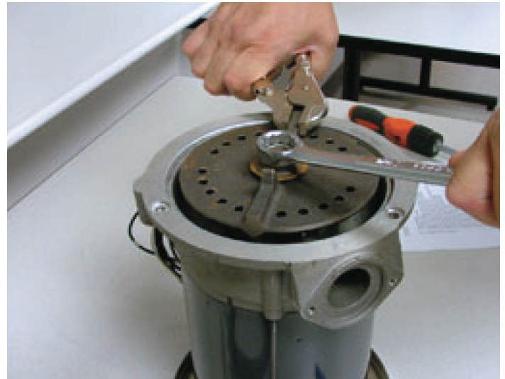
Figure 14. Rotating Shredder Nut
